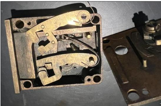
The lock was removed from the mausoleum and disassembled. It is a mortise lever lock, and likely dates from the 1920's. No manufacturer name is on the lock. The body and bolt are stamped with matching numbers. The manufacture of the lock mechanism is of high quality. All the parts fit together tightly. It is likely to have been hand made, and that's the reason for the numbers stamped into the parts.
