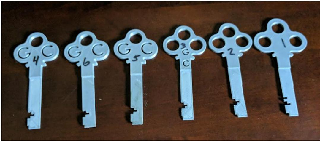
I ended up printing 6 keys. Starting with key 4, I could open the lock. From this point, I was able to make minor ( $\sim 0.010''$ ) tweaks to the model to make the key fit better and reduce the play. The last key opened the lock smoothly. Time to make it in brass!
