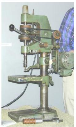
Joe Williams showed a taping machine which uses two belts from the motor to the spindle. When pulling the lever down, one belt drives the spindle containing the tap in a forward direction. When pulled up, the second belt drives the spindle in a reverse direction, backing the tap out. Joe also brought an assortment of various types of tapes including spiral point and a thread milling cutter.
