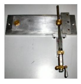
John Hoff showed the die shoe and component parts he fabricated to produce small brass boxes in a punch press.
