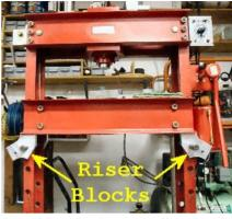
where full ram travel is required regardless of the table's vertical position. In the past, I've used shims to take up the gap between the ram's face and the presswork. But, that's both an unwieldy and dangerous practice. Commercially built presses are often fitted with a screw jack nested within the ram to make up any gap. Mine is home built, sans ram jack.
