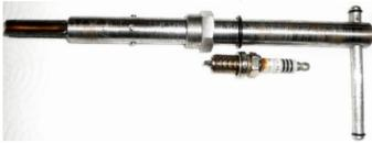
Dick Kostelnicek showed his 14-mm tap extension used to ream and collect the carbon buildup in a deeply recessed spark plug hole. The plugs were recessed six inches into an engine block and accessible through 0.90-inch diameter tubes. A large O-ring serves as a depth
