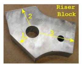
In order to refine the height adjustment of the table channels, I made four identical riser blocks from 1-inch thick aluminum that slip over the support pins (upper right photo). Each block has three flat faces that can support the table channels. The flats are spaced 120 degrees apart, and are located 1, 2, and 3-inches respectively above the top of
