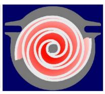
Dick Kostelnicek discussed the construction and operation of the scroll gas compressor. They are popular choices for split system residential air conditioners, where the condensing unit is placed outdoors while the evaporator and ventilation unit is inside the residence. Dick cut open a compressor, prior to the meeting, and passed around its upper and lower scrolls (third photo from left) so that all could observe the close tolerances attained during the manufacture of these compressors.
