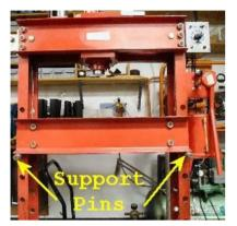
The height of the horizontal table channels on my H-frame hydraulic press could be adjusted only by 4-inch increments. The channels rest upon support pins placed in holes spaced along the vertical frame members (left photo). This 4-inch coarse adjustment makes it difficult to perform some tasks such as broaching,
