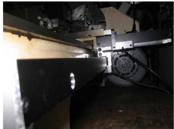
View down Z axis. Hole in cover is for access to mounting screw.
