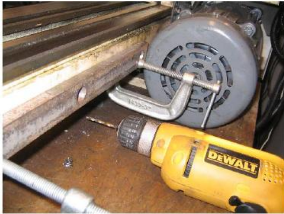
Using guide to assure hand drilled hole is perpendicular and in exactly the right place. Ended up being within 0.003"
