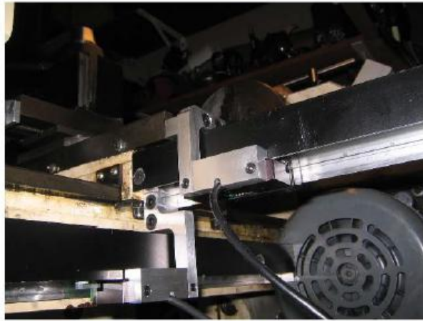
DRO read heads. Cables are repurposed USB.
