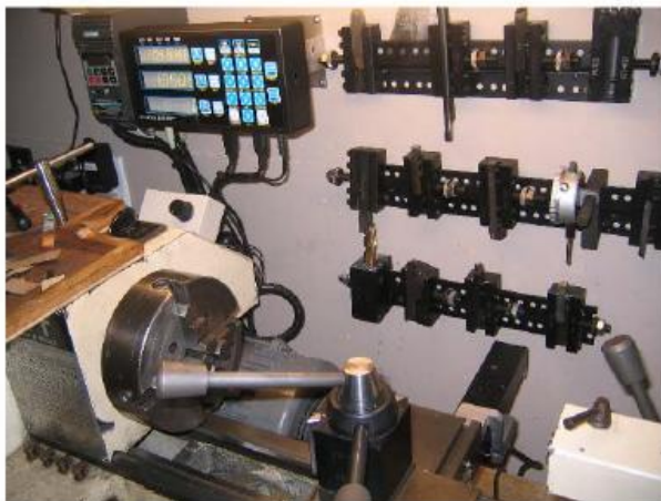
Overview of DRO and VFD
