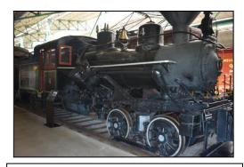
Photo 19: Heisler Vee Steam Engine
