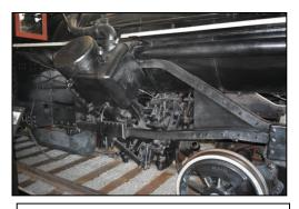
Photo 20: Close-Up of Twin Vee Steam Engine
