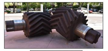
Photo 13: Pinion Gears
