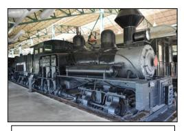
Photo 21: Shay Locomotive Engine and Tender
