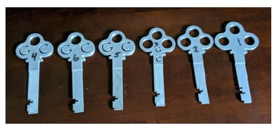
I ended up printing 6 keys. Starting with key 4, I could open the lock. From this point, I was able to make minor ( $\sim 0.010$ ") tweaks to the model to make the key fit better and reduce the play. The last key opened the lock smoothly. Time to make it in brass!
