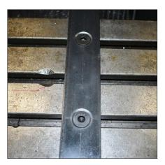
Rich Pichler exhibited stainless steel Rivet Nuts he used to repair a wheel mount on a utility cart. See photos below.
