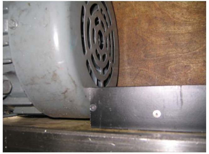
Z axis cover just touches motor housing
