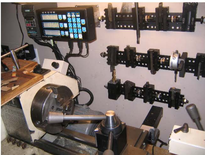
Overview of DRO and VFD
