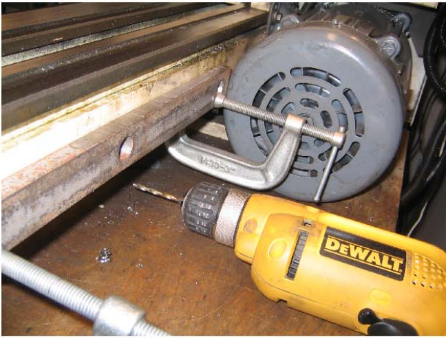
Using guide to assure hand drilled hole is perpendicular and in exactly the right place. Ended up being within 0.003"
